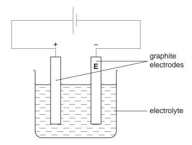
In experiment 1 the electrolyte was molten sodium chloride and in experiment 2 it was concentrated aqueous sodium chloride.
